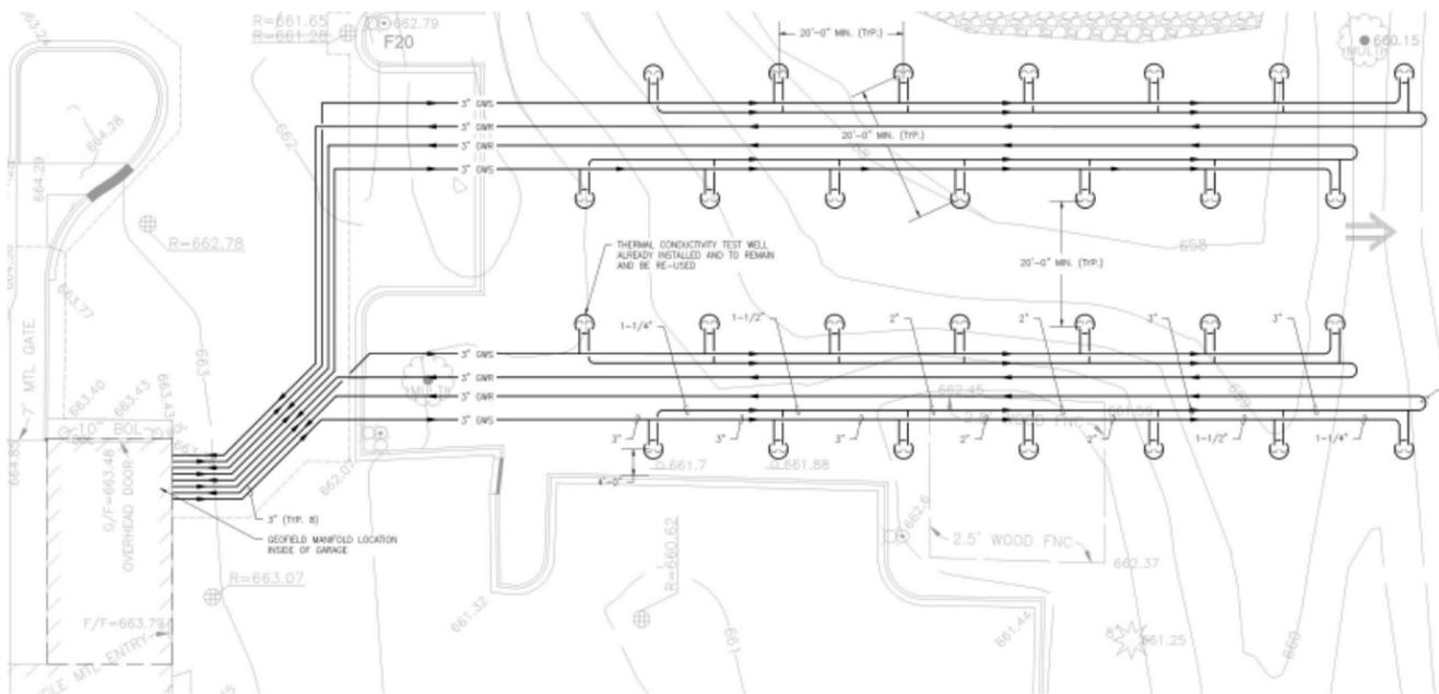
Geothermal Well-Field Layout
