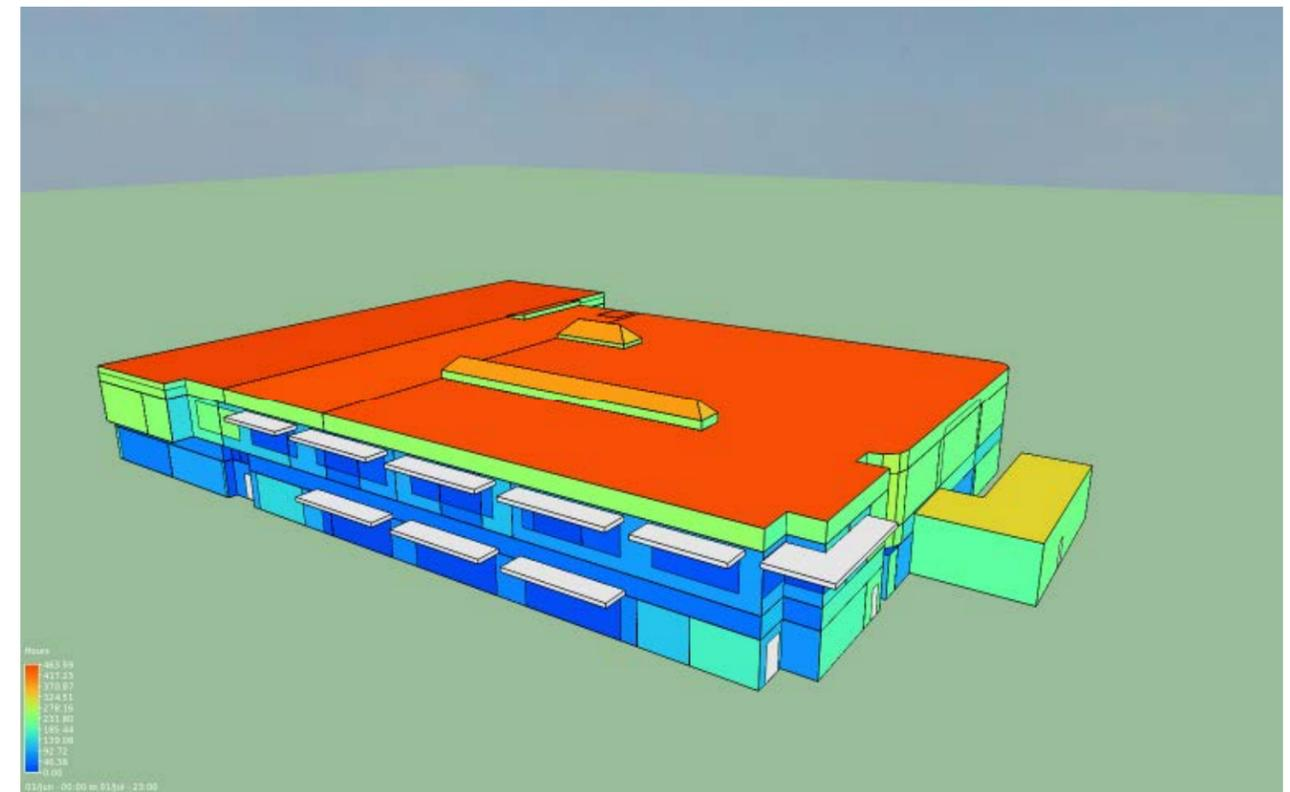
A 3-dimensional building model was constructed in the IESVE building analysis software, incorporating all building elements and thermal properties
